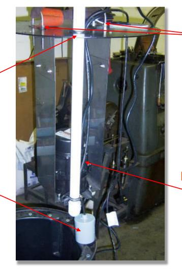
U-Bolts mount the system to the lid AND provide a convenient lifting means
