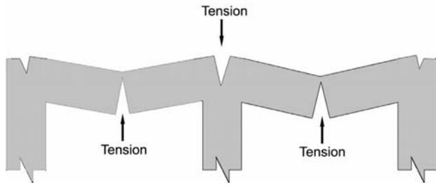
One of the things that happens to a concrete floor, or a masonry wall, is that they are subjected to forces that cause them to flex and bend. Examples
