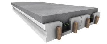
A carpenter friendly wood rib option is available. The wood rib can be removed after placement of concrete to be reused within the construction of the structure. Custom designs and pre-assembly are also options.
