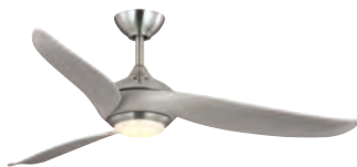
52" CONTE P250105-009-30 Brushed Nickel 20w LED, 3000K, 1865 lumens, dimmable 5037 CFM at high speed
