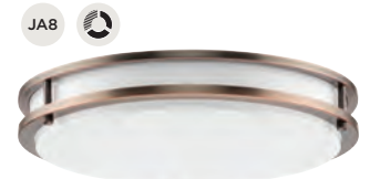
ABIDE LED P350275-174-CS Urban Bronze 14" dia., 2.83" ht. 19.8w integrated LED, 2700K/3000K/3500K/ 4000K/5000K, 90 CRI, 1162 delivered lumens.
