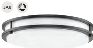
ABIDE LED P350275-31M-CS Matte Black 14" dia., 2.83" ht. 19.8w integrated LED, 2700K/3000K/3500K/ 4000K/5000K, 90 CRI, 1162 delivered lumens.
