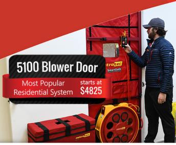
Test any residential house. Complete with a gauge, fan, ranges, connectors, & software. Auto & manual operation. Quick connect frame with extra crossbar for stability and gauge mounting. SmartCloth™ Wind Dampening cloth included.
