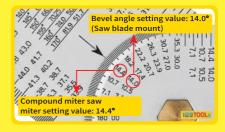
In this case, adjust the miter saw table angle to 14.4° and the bevel angle to 14.0°. Place the crown molding flat on the table (after double-checking whether this is to be a right- or left-side cut) and make your cut.
