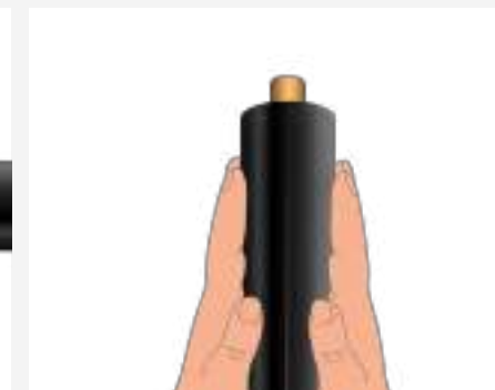
⑤ Reseal the tube around the pipe
