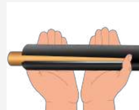
④ Allow adhesive to become tack-dry*
