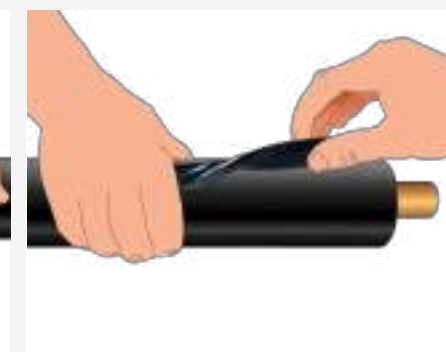
⑧ Secure seams using flame retardant tape
