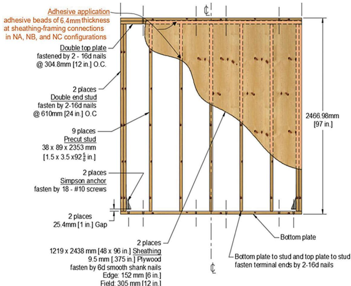
Figure 1 Schematic of the test specimen
