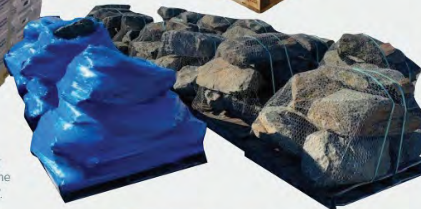
Palletized boulders wrapped or banded and wrapped in wire mesh.
