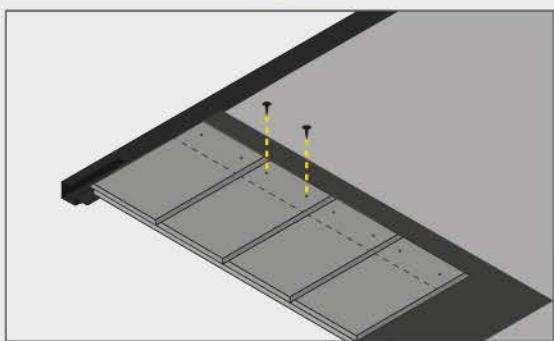
READYSLATE® is easily installed with nails. All individual slate tiles are predrilled to simplify the installation process.
