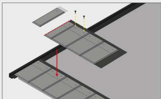
READYSLATE® slate tiles are marked with an overlapping line to ensure all modules are easily and correctly laid.
