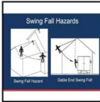
SWING FALLS FROM SINGLE POINT ANCHORS
