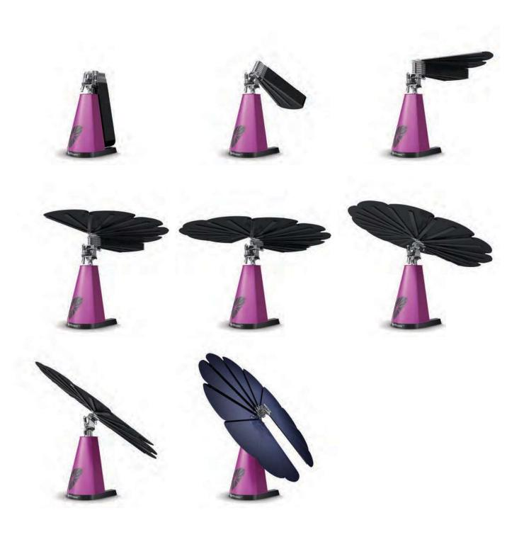
Astronomically controlled and movable across two axes: the circular solar modular fan constantly tracks the sun and always sets itself at an exact 90-degree angle to it, even when the sun is hidden behind clouds. The astounding result: up to 40% more output as compared to a conventional rooftop system, which receives optimum sunlight only for a few hours a day.
