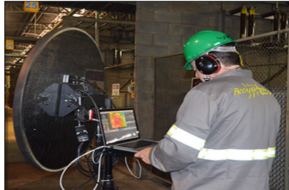
ARTVIS PINPOINTS NOISE SOURCE in 110dB AREA
