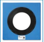
P-1000: **PLUMBING & HVAC** FLASHING PANEL Fits 10" sized pipes: copper, rigid, PVC, or ABS. Also fits 10" or 11" single wall sheet metal duct.
