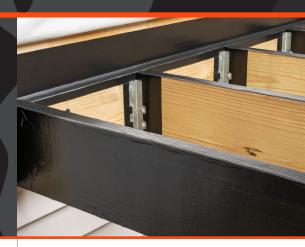
Protect and extend the life of your deck with CAMO Joist + Ledger Deck Tape. This self-adhesive butyl tape creates a waterproof membrane to protect wood deck framing against moisture, which can lead to rot. It self seals around fasteners, blocking the pathway of water into wood. Apply CAMO deck tape to the top of joists and ledger board, between joist hangers and ledger board, between rim joists and fascia, and between framing and joist hangers. Made in the USA.
