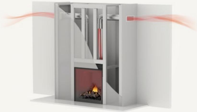
Operates without the need for electrical or blowers. Using a set of ducts, the heat is efficiently circulated around the room instead of blowing directly from the front of the fireplace. This is a silent system, which is ideal for spending quality time with loved ones watching a movie or reading. UHM lowers clearances for combustibles and allows for the safe installation of electronics above the fireplace.
