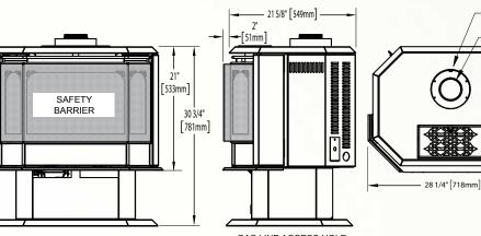
GAS LINE ACCESS HOLE LOCATED IN PEDESTAL REAR
