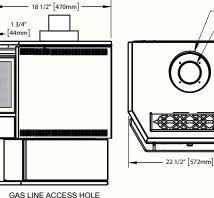
GAS LINE ACCESS HOLE LOCATED IN PEDESTAL BASE
