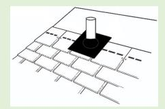
3. Install roof boot over vent pipe and Pro-Flash. Shingle remaining section
