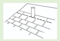
1. Install underlayment and shingles around vent pipe
