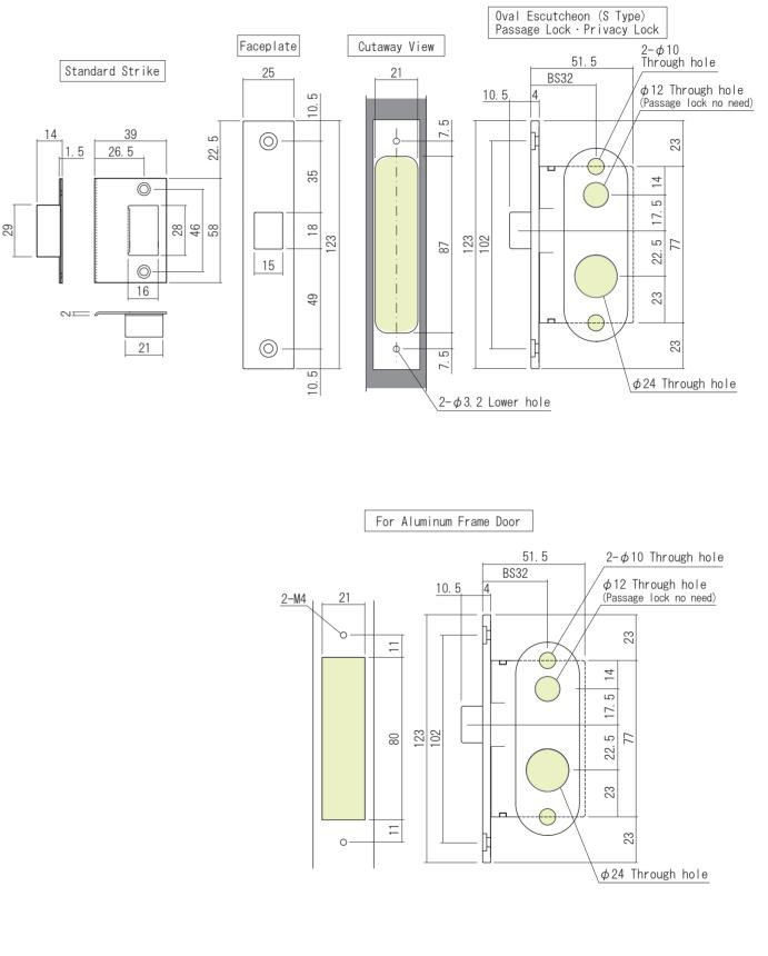
LU Lock Case Cutaway View
