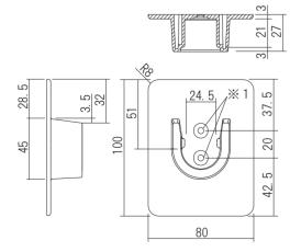
%1 You can use both double-sided tape and screws when installing the bracket to the wall.
