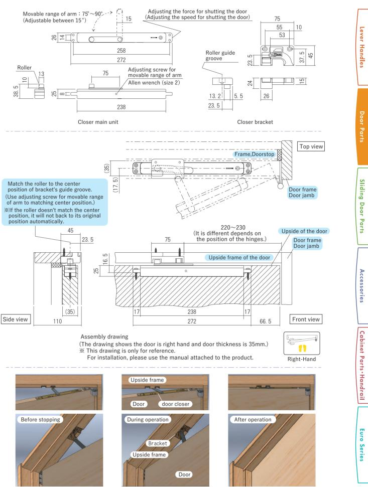
position of bracket's guide groove. (Use adjusting screw for movable range of arm to matching center position.) %If the roller doesn't match the center position, it will not back to its original position automatically.
