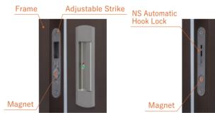
When the sliding door approaches the jamb (strike plate), the magnet will attract each other, then the hook will automatically strikes down and lock.
